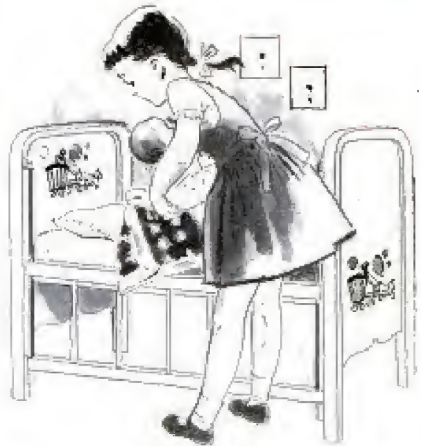
The two sides are identical and are made by driving pieces of 1/2-in. dowel through two rails made of 1 x 1-in. stock. Scrap of wood holds rails apart
